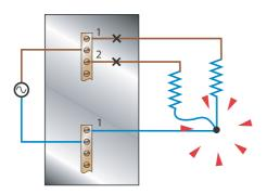
Lighting and control circuits are the most common examples where this practice is found. In these circumstances, the neutral conductor can become live when the conductor is disconnected, if a load is connected to that circuit.
