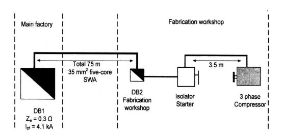
**Figure 1**Distribution arrangements for the three-phase compressor
